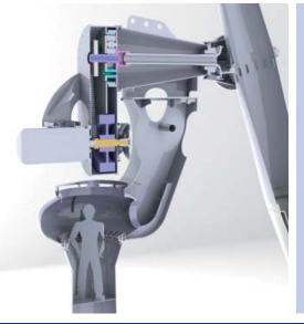
All the components that make up the power train have internal components that are rotating at different speeds and accumulate kinetic rotation energy that is much greater than that of the pendular unit itself.
