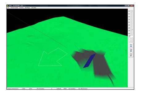
To refine the mesh locally, select the tracker and open the contextual menu to select the "Refine local mesh" option. This will open the following dialog box:
