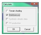
Now, as we did for the shading calculation, just change the hour of the day / day of the year to start the calculations. Whenever one tracker "hides" another, the second will become interfered, and automatically highlighted in red colour. The interfered tracker will keep the red colour until it would be free from interferences again.
