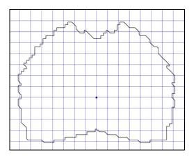
Obviously, a tracker's grid of 72 m x 55 m will produce no interference between trackers. However this grid is not necessarily the optimized solution. In this particular case, the minimum tracker's grid dimension that will not produce any interference is the square grid 46m (N-S) x 46m (E-W). The optimal grid dimensions are obtained by iterative checking.
