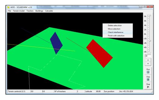
Select the *Check interference* option to highlight solar beams at interfered tracker corners. Interference occurs when a sun beam from one tracker corner intersects other tracker's or building's surface, as shown in the following screen:
