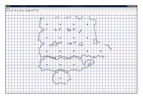
Shadows are irregular because terrain is not horizontal. As can be seen, the terrain under the three lower rows has a slope downwards South-East, therefore the N-S dimension of the shadows is shorter but the East part is longer than the West part. Terrain under the two upper rows has a slope downwards North-East.
