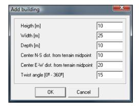
Enter the building dimensions -height, width, depth- and the building centre offset from the grid midpoint (similarly as for the tracker's grid). Also the building orientation angle with respect to the N-S direction can be defined. With the above data, the following building is created. A tracker has been manually deleted in that place.
