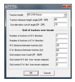
The input defines a grid of trackers of the selected ADES *Tracker model*. The fields are as follows:
