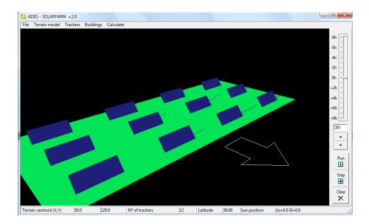
We have specified a tracker's grid of 3x8 units, however half of the trackers were out of the terrain limits according to the input grid dimensions. Solarfarm do not create trackers which coordinates are out the terrain mesh domain, therefore just 12 units are fitted.
