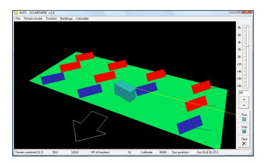
To solve this, we can mover trackers rows independently some meters away each other in the N-S direction, or delete all trackers and create a new tracker's grid.
