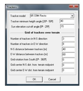
This grid produces minor interferences between days Nº 360 and Nº 36, which is an acceptable result for our particular criteria.
