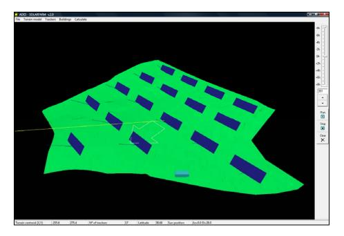
Now we perform some shading calculations -just for day numbers 351, 81 and 171- to obtain a first check. The result is shown in 2D view (terrain hided):
