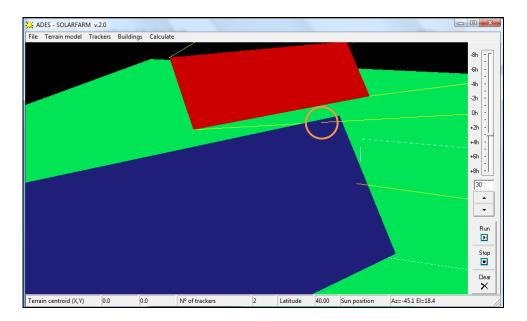
Interfered tracker will be partially shaded by the second one during this half hour. Because the "Example 1" case is symmetric with respect to South, the same interference will occur for the respective tracker in the period -3h to -3.5h (morning).
